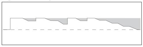
If the machine is switched on and there is no dispensing, the machine will be in energy safe mode after 30 min. The temperature of the boiler drops every 30 min. with 5 °C. If there is dispensing after 2 hours the machine is reactivated. The machine uses less energy if there is no dispensing or is left switched on.
