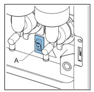
The on/off switch (A) puts the machine in the on/off position. The machine can still be charged after the machine is switched off. Unplug the machine to make sure that the machine is entirely uncharged.
