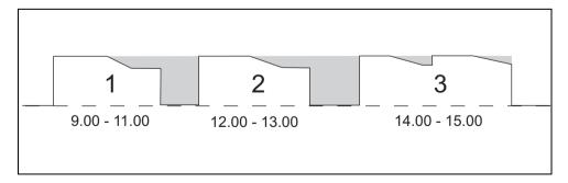
If the machine is switched on after being on standby and there is no dispensing, the machine will be in energy safe mode after 30 min. The temperature of the boiler drops every 30 min. with 5 °C. If there is dispensing after 2 hours the machine is reactivated. The machine uses less energy if there is no dispensing or is left switched on.
