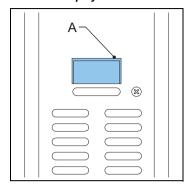
The display shows technical malfunction with error codes. The display also provides additional user information or warnings.
