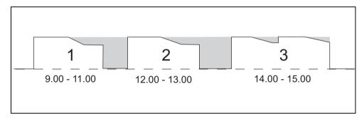
If the machine is switched on after being on standby and there is no dispensing, the machine will be in energy safe mode after 30 min. The temperature of the boiler drops every 30 min. with 5 °C. If there is dispensing after 2 hours the machine is reactivated. The machine uses less energy if there is no dispensing or is left switched on.
