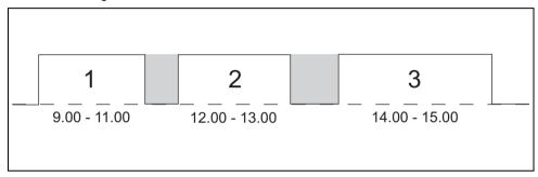
The machine switches on at 9.00/12.00/14.00 automatically. The machine is on standby at 11.00/13.00/15.00. During standby mode the control panel is switched off and the boiler temperature drops to the set boiler temperature.
