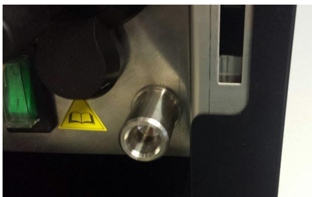
Hot water coupling
