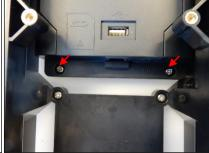
8. Press the glass panel and Optilight panel together and hold it for a couple of seconds, it should be stuck now.
