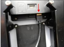
4. Remove 6 screws, hold the panel!
