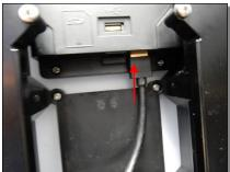
12. Put the cable back into its original position
