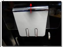
3. Remove the metal cover plate at the inside of the machine door, remove the wires.
