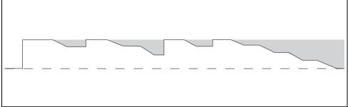
If the machine is switched on and there is no dispensing, the machine will be in energy safe mode after 30 min. The temperature of the boiler drops every 30 min. with 5 °C. If there is dispensing after 2 hours the machine is reactivated. The machine uses less energy if there is no dispensing or is left switched on.
