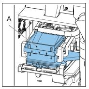
The brewer (A) receives the product from the grinder. The product is made by vacuuming hot water through the filter. The brewer piston transfers the product to the outlet. A wiper transfers the residue to the waste bin.
