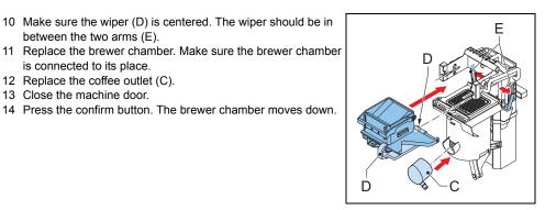
Replacing the filter
