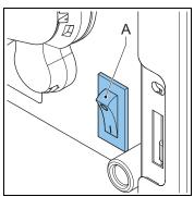
The on/off switch (A) puts the machine in the on/off position. The machine can still be charged after the machine is switched off. Unplug the machine to make sure that the machine is entirely uncharged.
