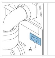
The on/off switch (A) puts the machine in the on/off position. The machine can still be charged after the machine is switched off. Unplug the machine to make sure that the machine is entirely uncharged.
