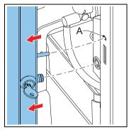
The door switch (A) automatically switches off the machine when the door is opened.
